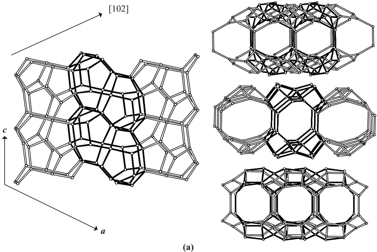
Figure 5. (a): Fused channel intersections in **HEU** viewed along  $b$  (left), and (from top right to bottom right) along  $a$ ,  $c$  and  $[102]$ . [Figure 5 is continued on next page]
