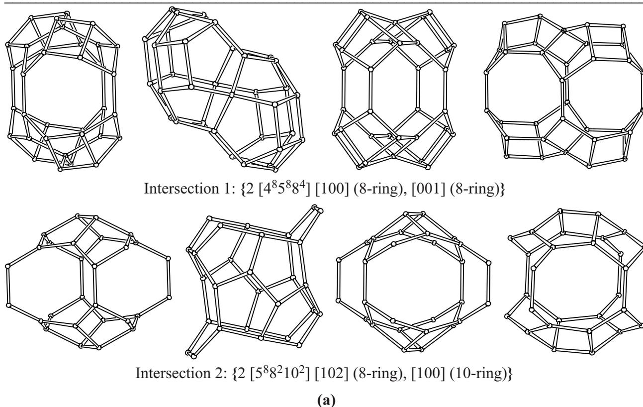
Figure 4. (a): Intersections of channels in **HEU**, with **pore descriptors**, viewed (from left to right) along  $a$ ,  $b$ ,  $c$  and  $[102]$ . [Figure 4 is continued on next page]
