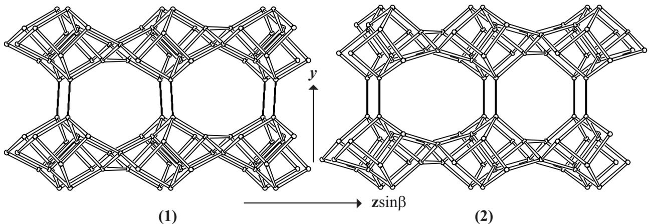
Figure 2. Connection mode (1) in **RRO** and connection mode (2) in **HEU** viewed along  $x$ .
